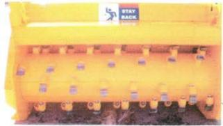
Tip to tip cutting diameter of the rotor is 28 inches (711 mm). The rotor is fitted with carbide tip heat treated steel cutters which are quick change, pocket mounted incorporating cutter overlap.
