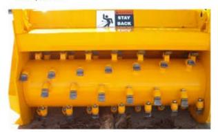
Tip to tip cutting diametere of the rotor is 28 inches (711 mm). The rotor is fitted with carbide tip heat treated steel cutters which are quick change, pocket mounted incorporating cutter overlap.
