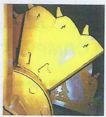
USE PADDLE AERATOR W/ OPTIONAL SPADE HI-CARBON OR CARBIDE TEETH FOR INSITU MILLING, WINDROW FORMATION & AERATION
